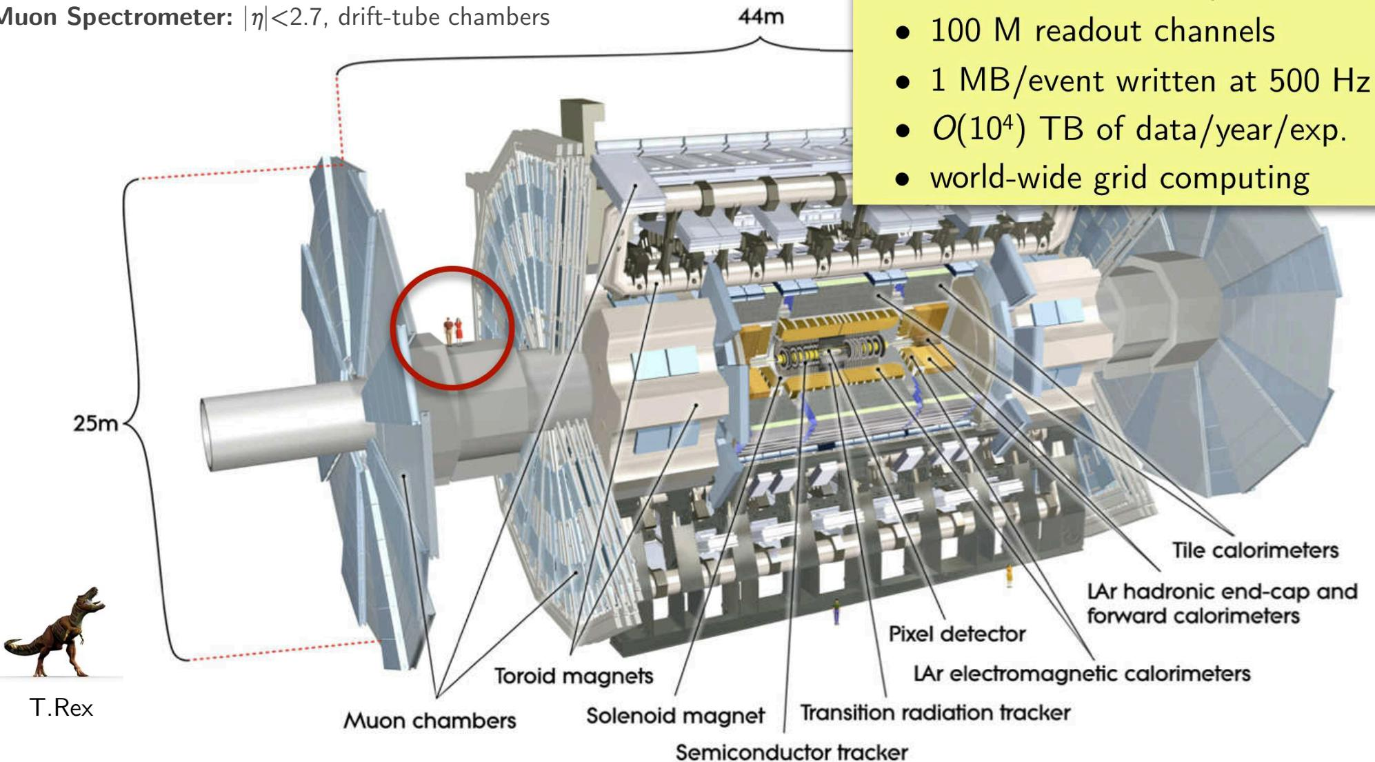
Tracking:  $|\eta| < 2.5$ ,  $B=2\text{T}$ , precise tracking and vertexing, Si pixels, strips, and TRT straws, TR electron ID
