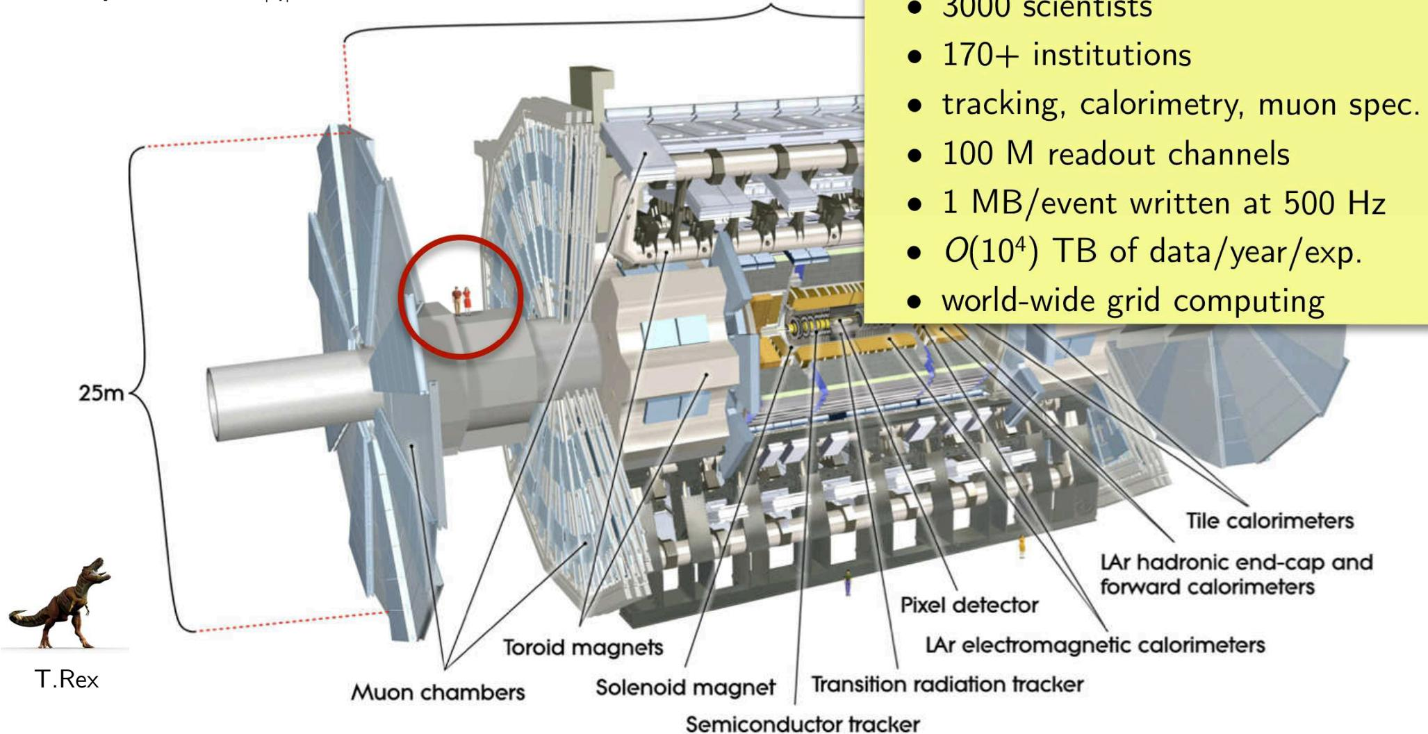
**Tracking:**  $|\eta| < 2.5$ ,  $B=2\text{T}$ , precise tracking and vertexing, Si pixels, strips, and TRT straws, TR electron ID
